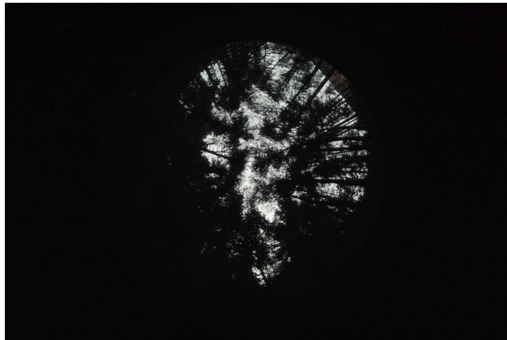
Figure 6. A pre-treatment hemispherical photo for a stream that will receive a gap treatment in the Valsetz block. Photos were taken by placing a camera on a tripod facing up in the stream, leveling the lens, then taking a photo of the canopy overstory.
